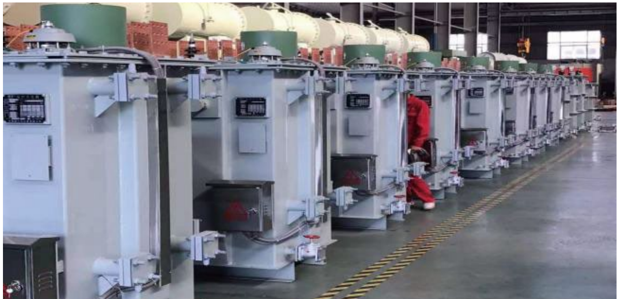
▲ 10KV FURNACE TRANSFORMER
