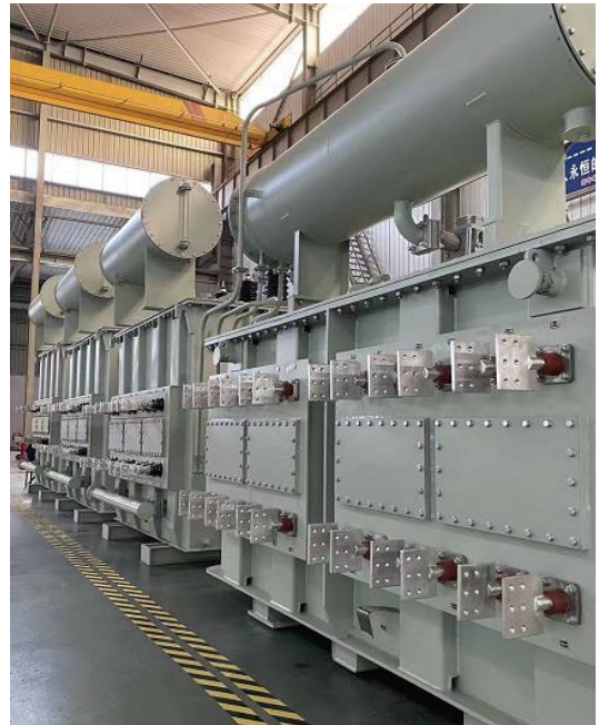
>35kV furnace transformer
